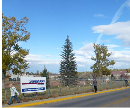
Sidewalks without buffers create less comfortable and safe walking conditions
